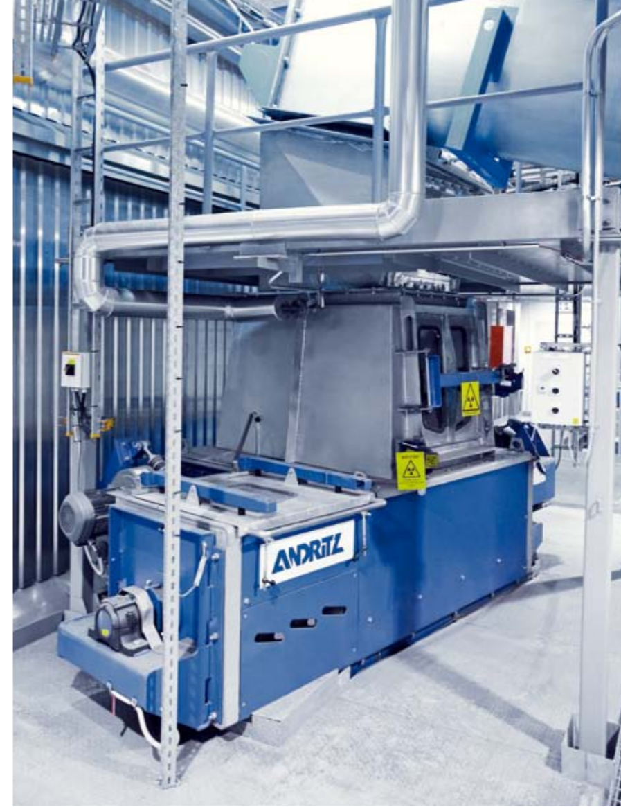
▲ The balancing bin, proportioning the biomass fuels, is the most critical part of the fuel feeding system.
