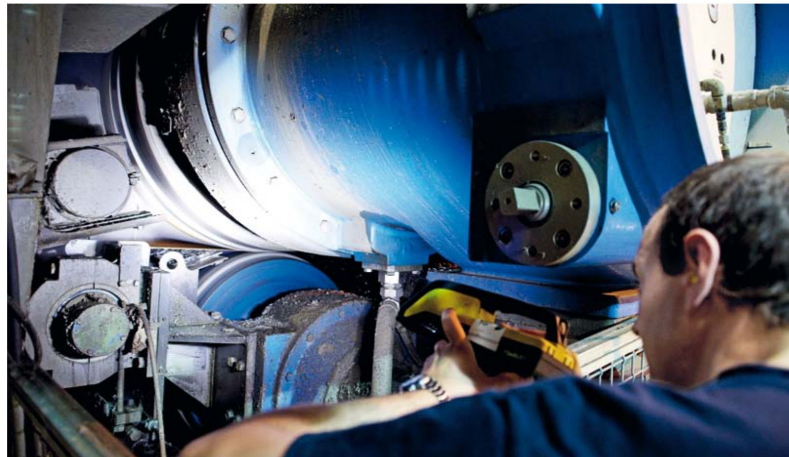
Alexis Zenner of VPK inspects the first nip between the press roll and suction press roll of the PrimePress Trix . ▼
