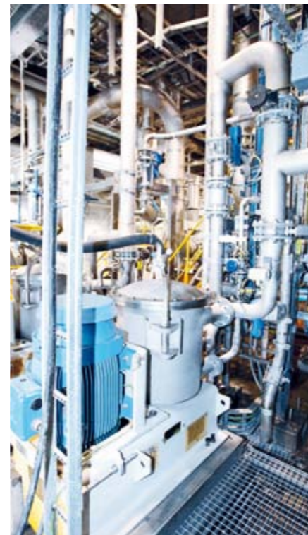
▲ As part of the stock prep package, ANDRITZ also delivered the ModuScreen broke screening system and the protection screens.
