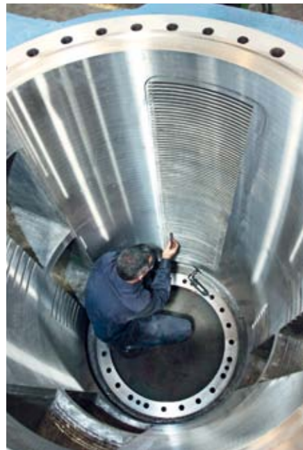
▲ Craftsmen at work. Rebuilding and upgrading feedline equipment for continuous digesters.
