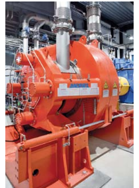
▲ The use of LC refining for the secondary stage or rejects processing contributes to overall energy savings. Shown above is the world's largest LC refiner – the TwinFlo 72.
