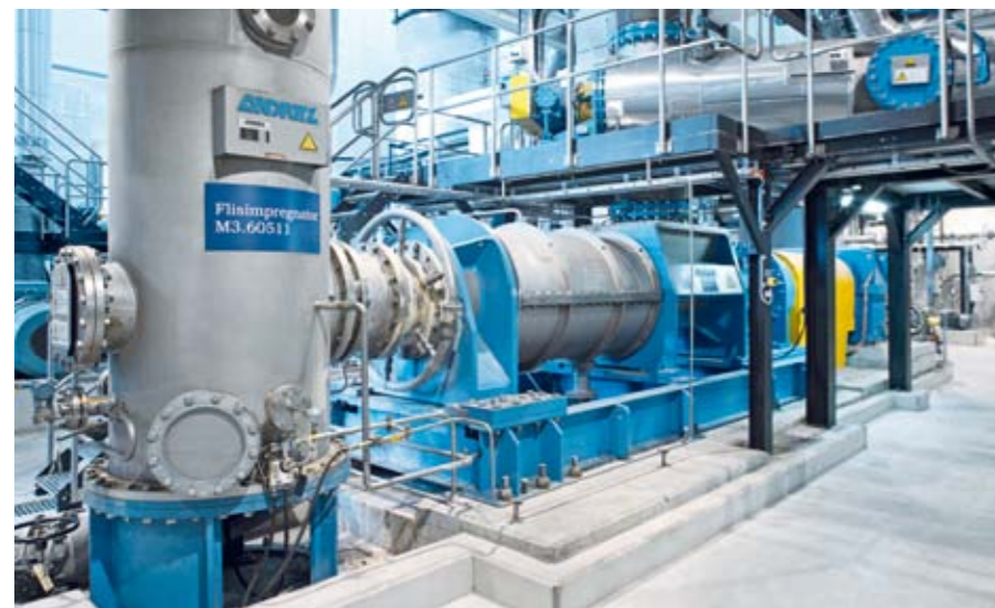
The MSD Impressafiner (shown below) and a Fiberizer delaminate the wood chips into loose fiber bundles which are perfect for targeted chemical treatment. ▼
