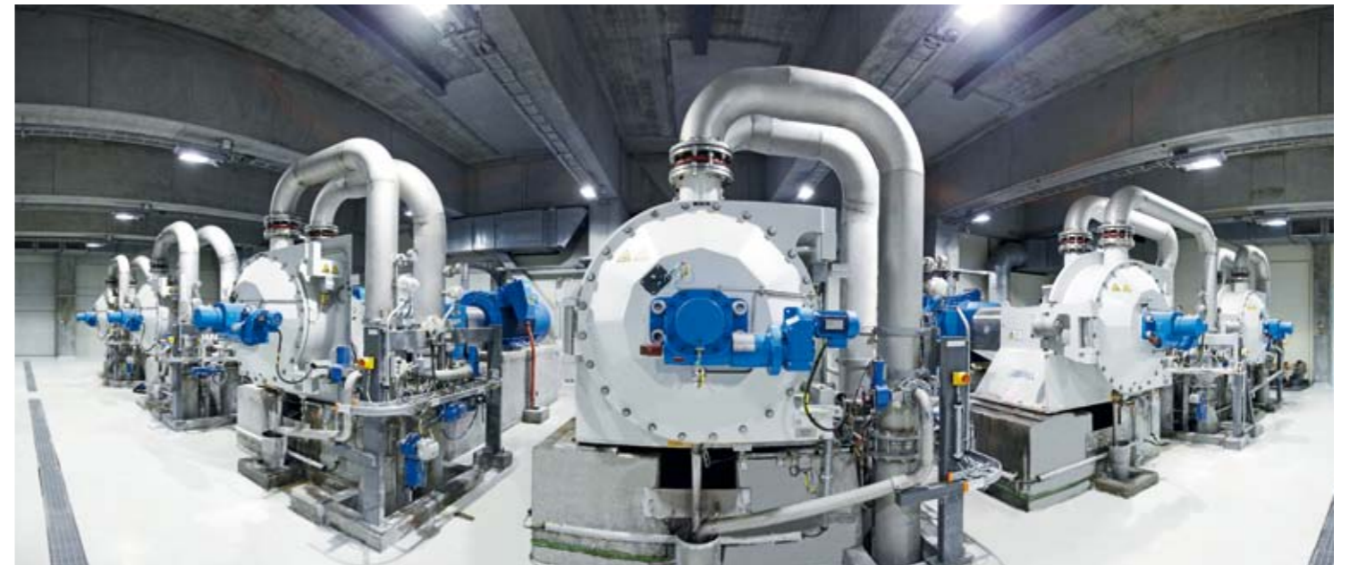
▲ A view of the TwinFlo refiners (eight for hardwood and two for softwood) delivered by ANDRITZ for PM4's stock preparation.
